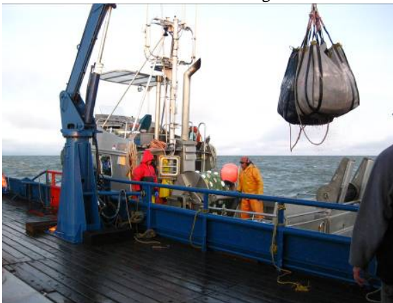
Fish are transferred from fishing boats to tenders in brailer bags or are pumped through large hoses.
